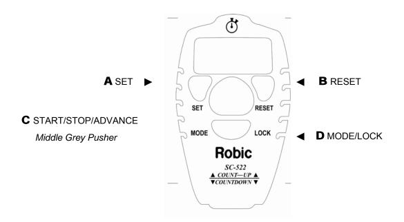
Pusher A: "SET" Pusher B: "RESET" Pusher C: Start/Stop/Advance (Middle Grey Pusher) Pusher D: "MODE LOCK"
